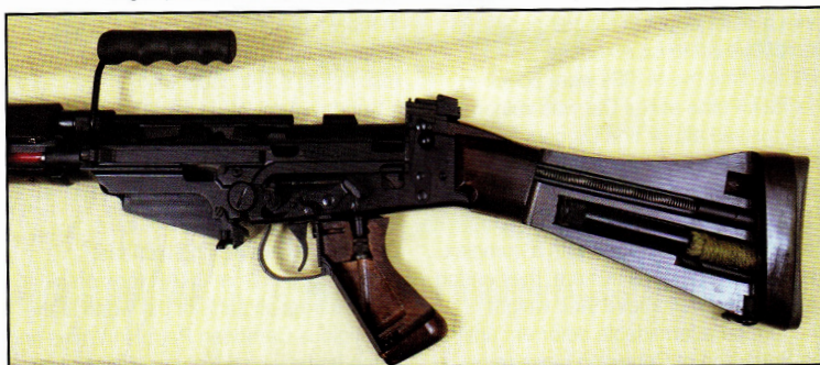
A Lithgow factory cutaway example of an Australian L1A1 showing the return spring for the bolt carrier's "rat tail" and the oil bottle and pull through stowage in the butt stock.
